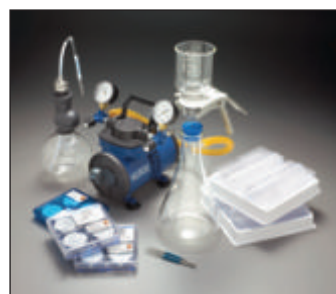
Membrane filtration system
